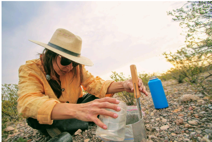
Figure 5: CRI Project Manager Garcia measures the infiltration rate of arid rocky soils.
