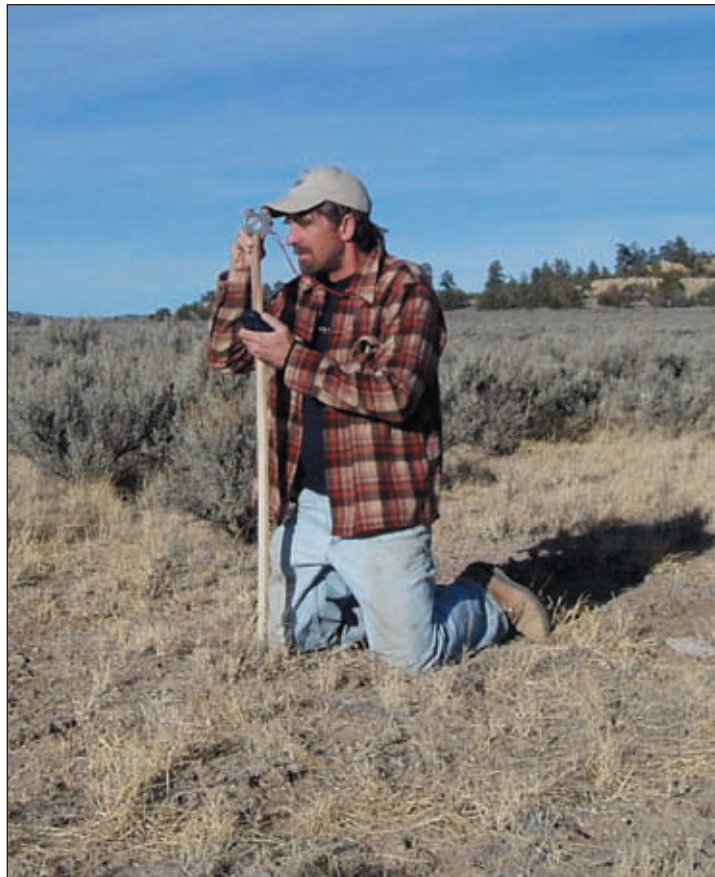
Photo VI-3: Using a clinometer to measure the percent slope of a landscape.
